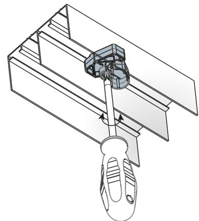
Stopper limits and stops the motion of the cabinet door.
