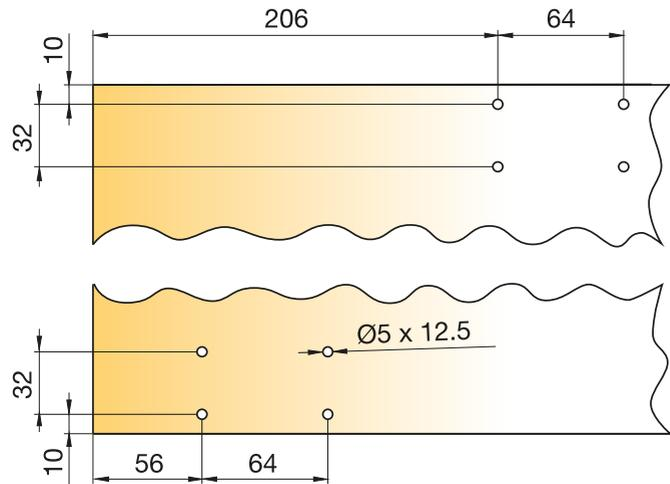
Top and bottom carriage drilling positions
