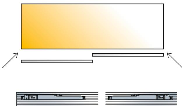
Mount Titusoft SD100s on top rail on both sides of the cabinet (1 mechanism per door).
