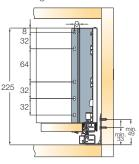
Installation dimensions for the front panel
