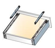
Position both SDWD-T mechanisms on the bottom of drawer
