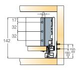
Installation dimensions for the front panel
