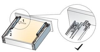
Allign SDWD-T mechanisms with drawer lip and push to the front panel
