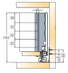
Installation dimensions for the front panel
