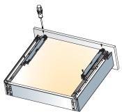
Screw-on both mechanisms
