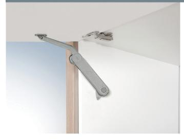
Combine with soft close hinges for smooth operation. Weight capacity: Adjustable to 20kg Cabinet height: 300 - 600mm 32mm standard drilling Minimum cabinet depth: 200mm
